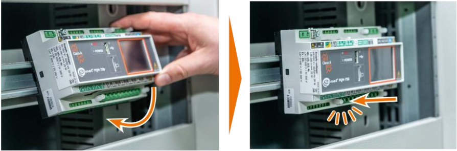
Fig. 5 Mounting the analyzer on the DIN EN 60715 35 mm rail.
