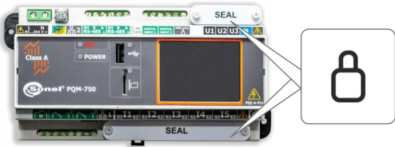
Fig. 7. Sealing of the measurement terminals.
